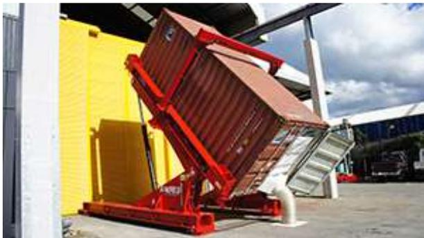
A-Ward's unique MiTilt™ unloader eliminates the need for scarce and expensive tilting trailers. Whether your material is being unloaded through a grate, over an edge, or directly in the ground, the MiTilt™ enables faster, cleaner and safer unloading.
