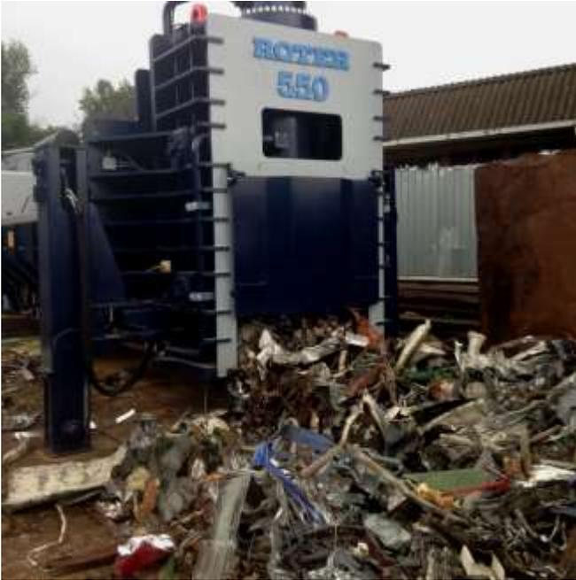
RR series shear/balers for scrap metal are the best solution to **compact and shearing all types of steel and ferrous and not ferrous metals.**
