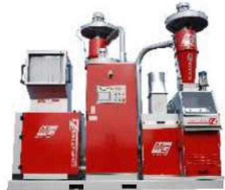
The MG 380 VZT is a complete technological system for copper and aluminum recovery from electric cables and other waste materials. 99.9% of clean recovered material can be achieved using the technology of the air separation table after the grinding and pulverising process.
