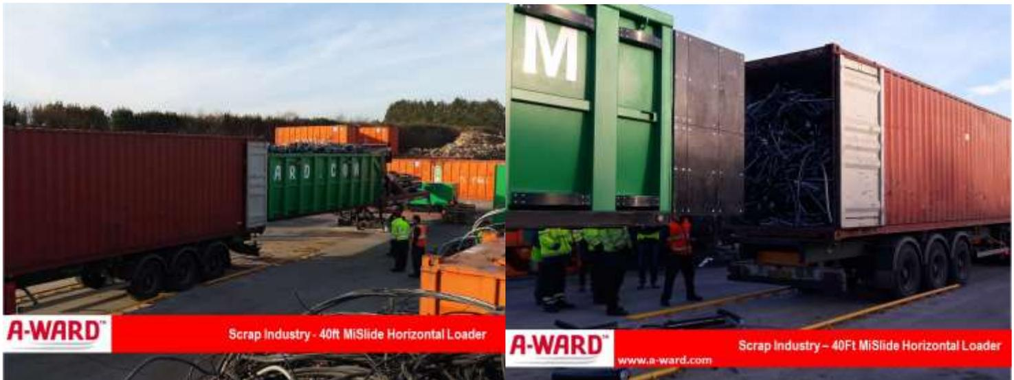
The Mi-Slide from A Ward allows you to load scrap, or any other commodity or waste in to the charging bay, this allows you to pre weigh the load before the container even arrives. The container truck simply backs the open container on to the Mi-Slide until it reached the end. The Mi-Slide then powers the load forward in to the container and pushes the truck forward until the container is loaded.
