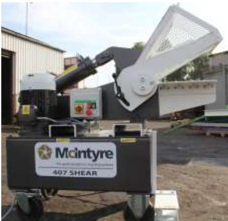
The 407 is basically the same machine as the 320 but with a different pump and larger jaws, enabling it to do larger cuts
