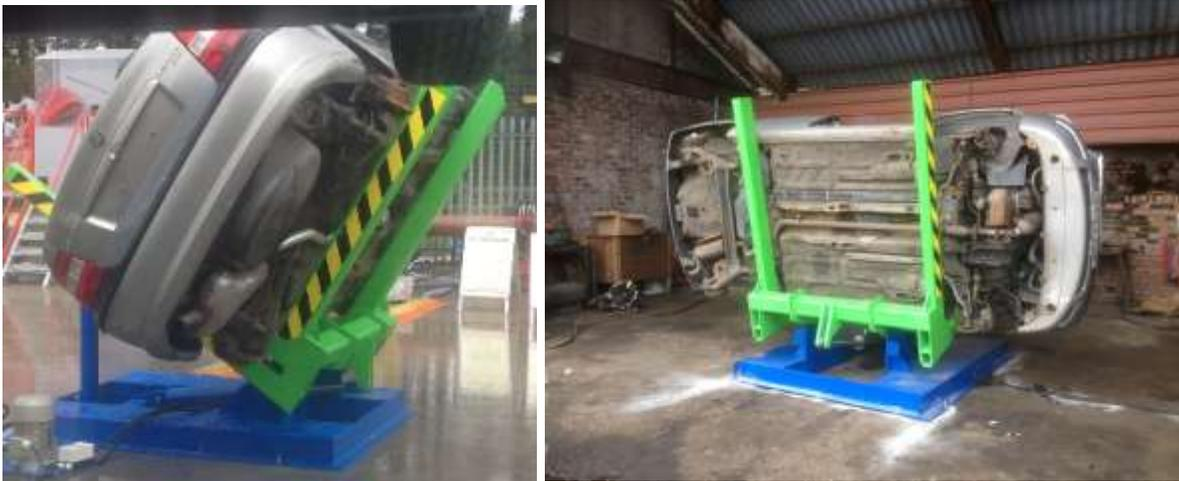
The side tip vehicle stand tilts the vehicle back hydraulically for the easy recovery of parts from the underside of the vehicle. The unit supports the vehicle to prevent it falling backwards off the stand. It makes the task of accessing under the vehicle much easier and quicker than putting it on a lift.
