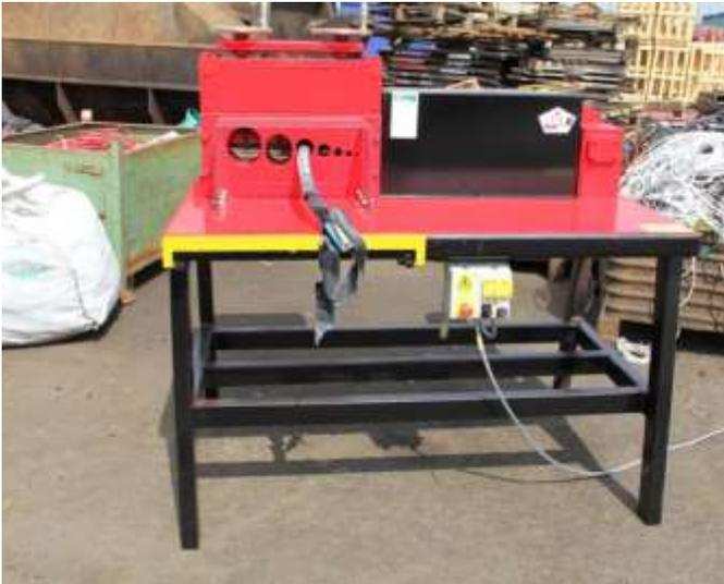
The ES5000 cable stripper will handle most heavy-duty cables including armored and multi-core. It's easy to use and can process cable from 1/8" up to 4" diameter at speeds of up to 138 feet a minute. Adjustment is simple and there is no need for constant setting changes to suit different material sizes.
