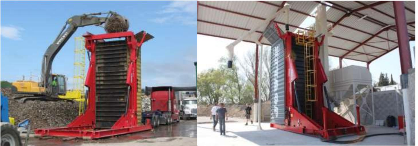
MiTilt™ is a revolutionary tilting container loader that allows you to gravity-load your containers to maximum capacity. It combines patented tilting technology with a choice of four different bodies or frames, to suit your type of operation. The MiTilt™ is safely controlled by a single operator and allows you to weigh the container during loading and maximize the fill weight.
