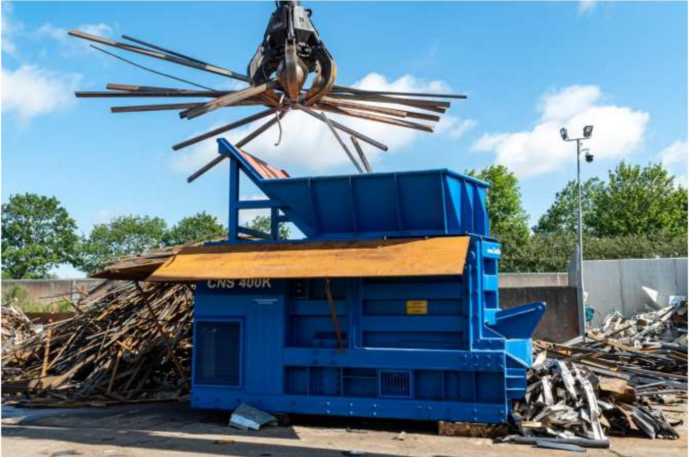
The ZDAS CNS400K Horizontal Scrap Shear is designed to shipping container dimensions for easy transport. It is a self contained machine with a built in diesel engine powered hydraulic power pack.
