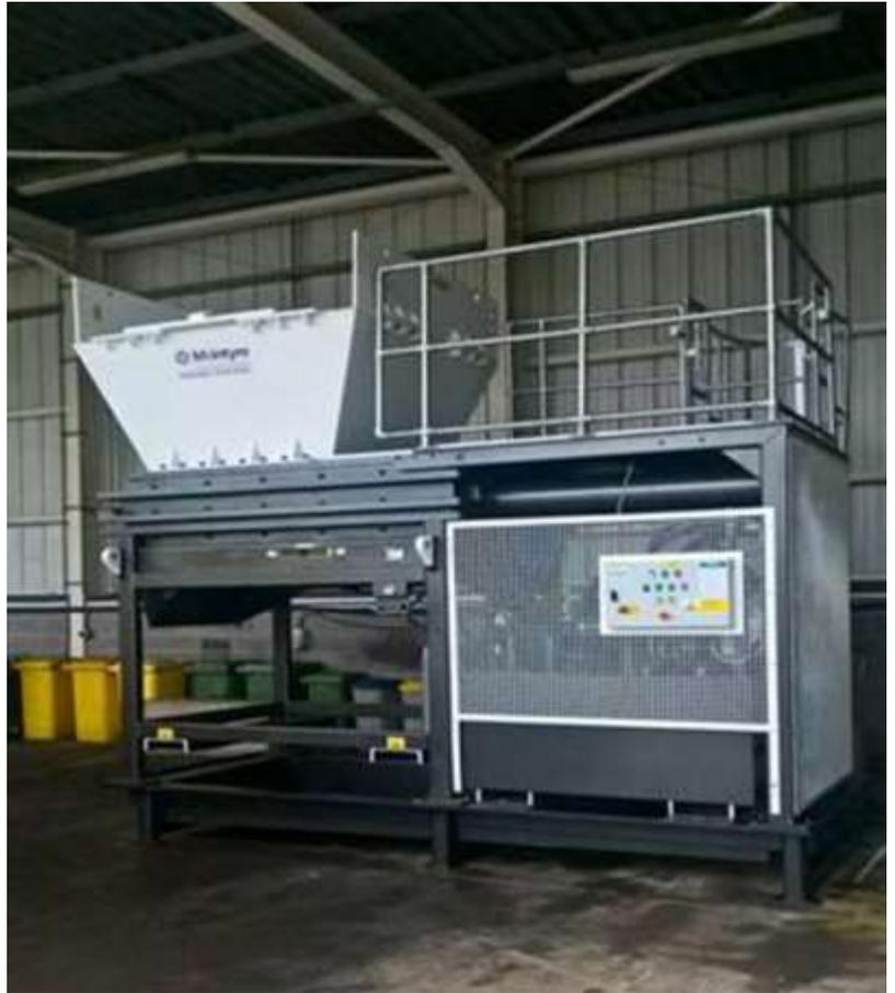
The unit comes with a complete oil collection tray that sits under the whole machine. Oil is collected on the outlet chute and a couple of other areas and can be directed to a storage tank if required. This keeps the area as clean as possible when dealing with this type of product.
