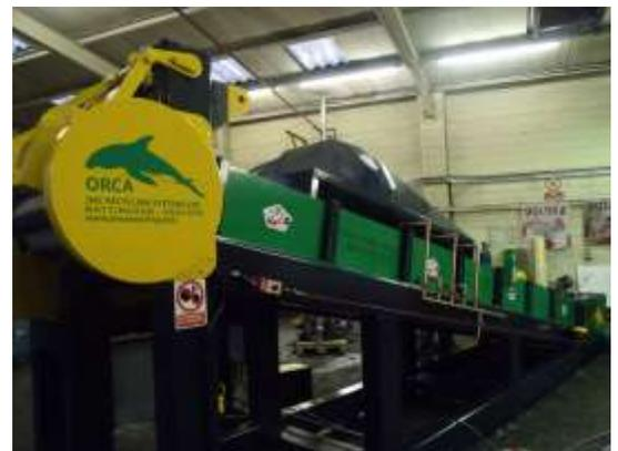
The Orca can have either 92 or 120 moulds depending on your requirements. It is capable of producing up to 14,000 lbs an hour depending on its mold format
