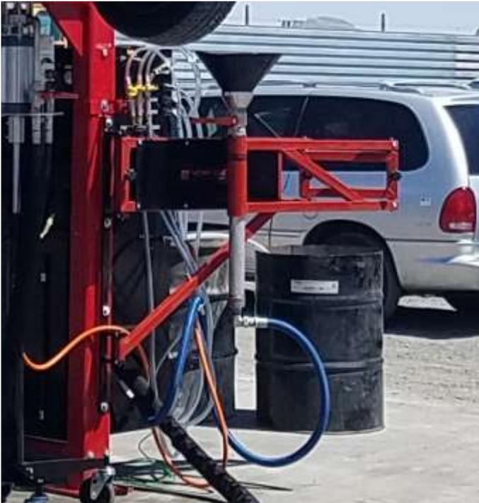
The differential / rear axel drainer arm is designed for yards wishing to recover the oil from rear axels before crushing or shredding the vehicle.
