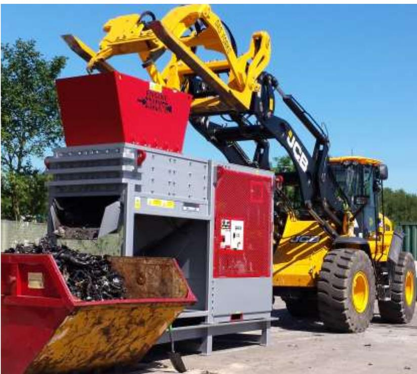
An Engine Cracker being loaded with an SAS Scorpion Engine Puller.
