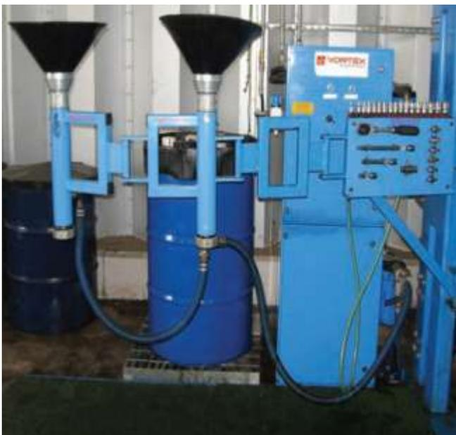
An easy to use system that will quickly drain used engine and transmission oils then pump the oil away to storage tanks. This avoids moving open tanks or drainers on wheels around the yard to empty them.
