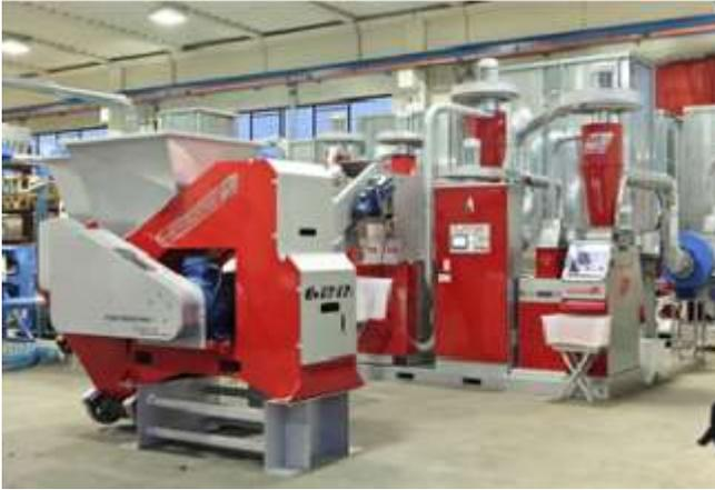
The MG 220ZVT is a complete technological system for copper and aluminum recovery from electric cables and other waste materials. 99.9% of clean recovered material can be achieved using the technology of the air separation table after the grinding and pulverising process.
