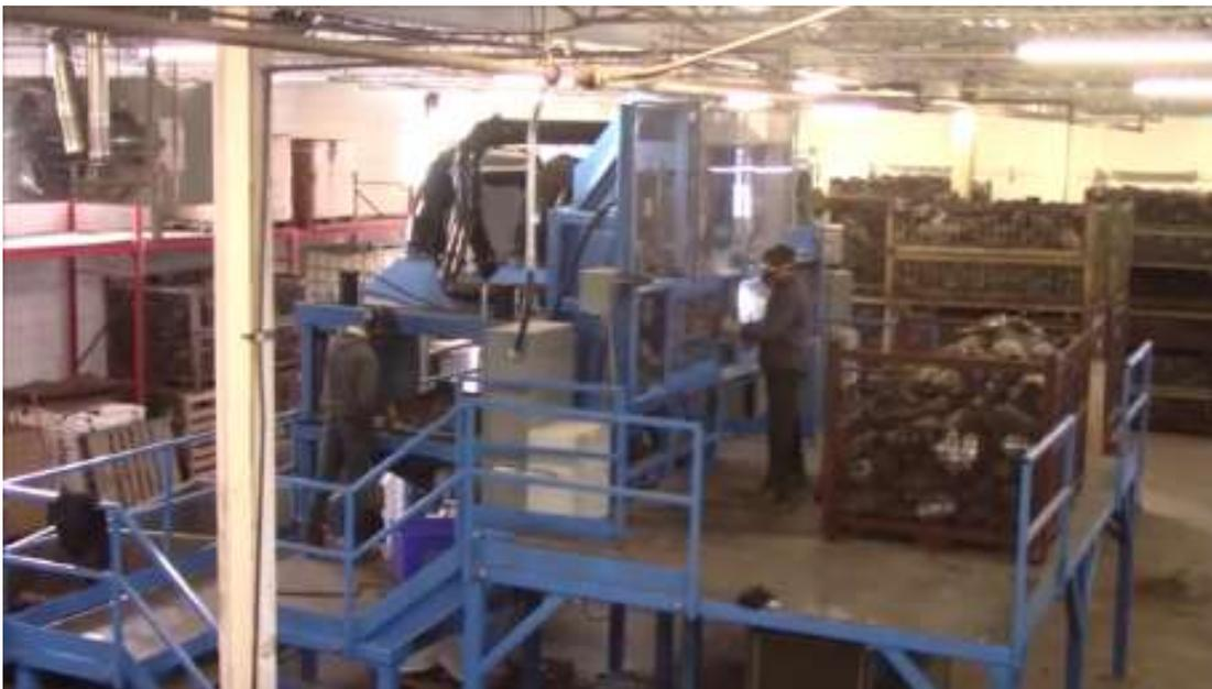
The double blade guillotine with 4 or 6 opening stations is capable of processing between to 400 & 500 converters an hour and has powerful dust collection systems to ensure none of the valuable dust is lost.
