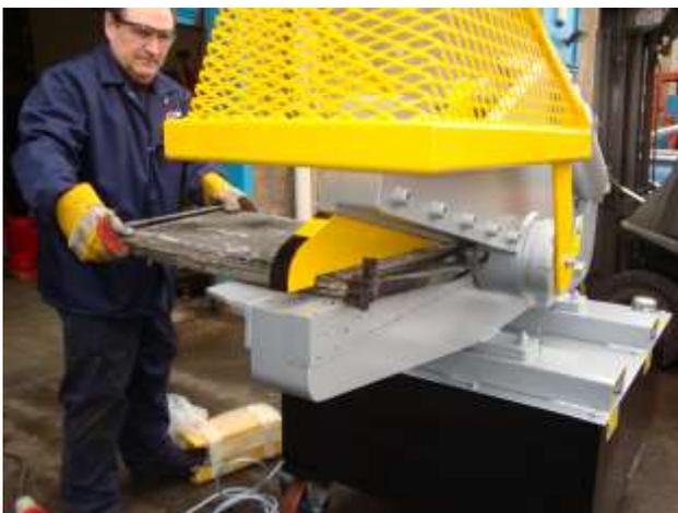
The 600 shear is large enough to trim radiators in a single cut, it comes with options for a cat shear and a hydraulic hold down as shown.
