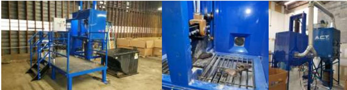
The single Cat Guillotine, capable of processing 60 converters per hour
