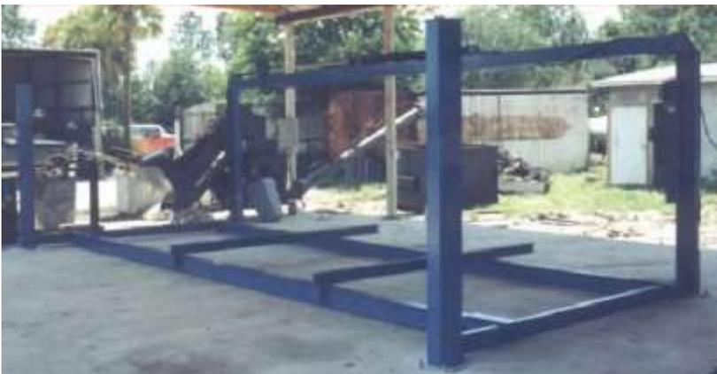
The TSL9SL is an economical side load lift with a 276" opening on long side for loading
