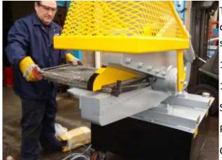
The 600 shear is large enough to trim radiators in a single cut, it comes with options for a cat shear and a hydraulic hold down as shown.
