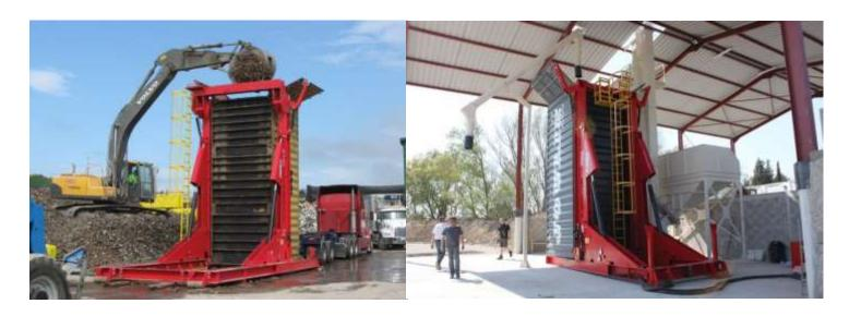
MiTilt<sup>TM</sup> is a revolutionary tilting container loader that allows you to gravity-load your containers to maximum capacity. It combines patented tilting technology with a choice of four different bodies or frames, to suit your type of operation. The MiTilt<sup>TM</sup> is safely controlled by a single operator and allows you to weigh the container during loading and maximize the fill weight.
