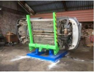
The side tip vehicle stand tilts the vehicle back hydraulically for the easy recovery of parts from the underside of the vehicle. The unit supports the vehicle to prevent it falling backwards off the stand. It makes the task off accessing under the vehicle much easier and quicker than putting it on a lift.
