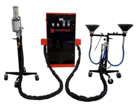
Vehicle top and bottom de-pollution station that can be used in conjunction with lifts or fixed stands Four 1" double diagram pumps with strainers
