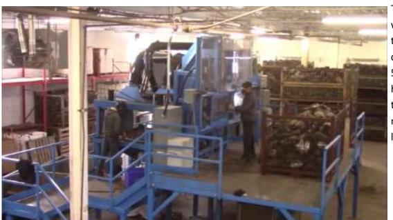
The double blade guillotine with 4 or 6 opening stations is capable of processing between to 400 & 500 converters an hour and has powerful dust collection systems to ensure none of the valuable dust is lost.
