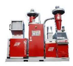
The MG 380 VZT is a complete technological system for copper and aluminum recovery from electric cables and other waste materials. 99.9% of clean recovered material con be achieved using the technology of the air separation table after the grinding and pulverising process.
