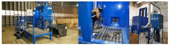
The single Cat Guillotine, capable of processing 60 converters per hour
