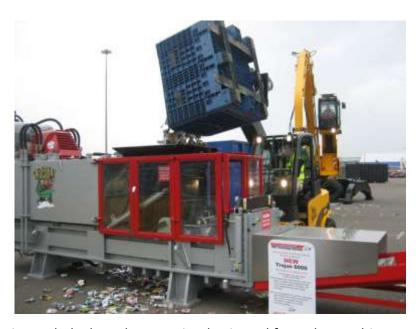
Such dense bales means that no tying or strapping is needed. The cubes are simply ejected from the machine and ready for transportation. The Trojan is a totally automatic system and only requires to be fed material. Once started, the operator is free to load or unload the machine as well as attend to other aspects of your business.
