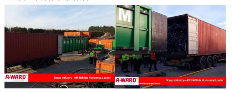
The Mi-Slide from A Ward allows you to load scrap, or any other commodity or waste in to the charging bay, this allows you to pre weigh the load before the container even arrives. The container truck simply backs the open container on to the Mi-Slide until it reached the end. The Mi-Slide then powers the load forward in to the container
