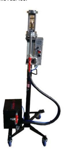
The Vortex Fuel Tool powered by compressed air punches through the fuel tank.
