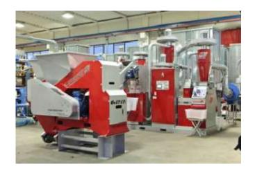
The MG 220VZT is a complete technological system for copper and aluminum recovery from electric cables and other waste materials. 99.9% of clean recovered material con be achieved using the technology of the air separation table after the grinding and pulverising process.
