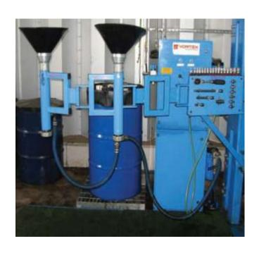
An easy to use system that will quickly drain used engine and transmission oils then pump the oil away to storage tanks. This avoids moving open tanks or drainers on wheels around the yard to empty them.
